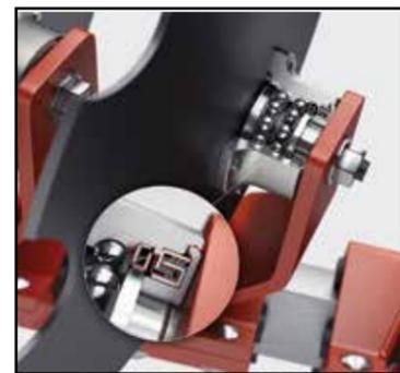
"Alongside high-performance bearing technology, Agri Disc hubs are equipped with a highly effective sealing system for robust protection against extreme condition applications. This comprehensive system is a combination of labyrinth and contact seal designs, which serves to prevent both the ingress of contaminants and the escape of grease."
